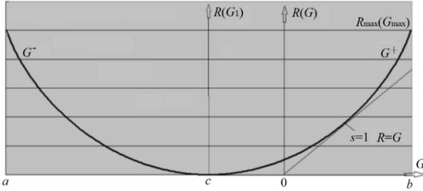
Fig. 2. The  $R(G)$  function of a binary source (for details, see [12]). As  $s=1$ ,  $R=G$ , which implies that the semantic channel matches the Shannon channel;  $R_{\max}(G_{\max})$  at the top-right corner means that the Shannon channel matches the semantic channel so that both  $R$  and  $G$  are at their maxima.
